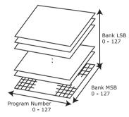
This is a 3D image of the expanded program change system with the MSB and LSB. To use these efficiently and correctly, refer to the operation manual of any external MIDI sound modules that are connected to the MP5.
